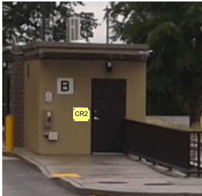
**Door #2 – Weight Station** = Add Card Reader (1) , REX, D/C, Electrified Strike, Controller panel (under desk or on wall). Change hardware to Storeroom function
