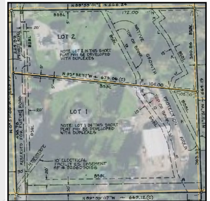
Example of Protective Easement on Individual Lot and Unpermitted Construction
