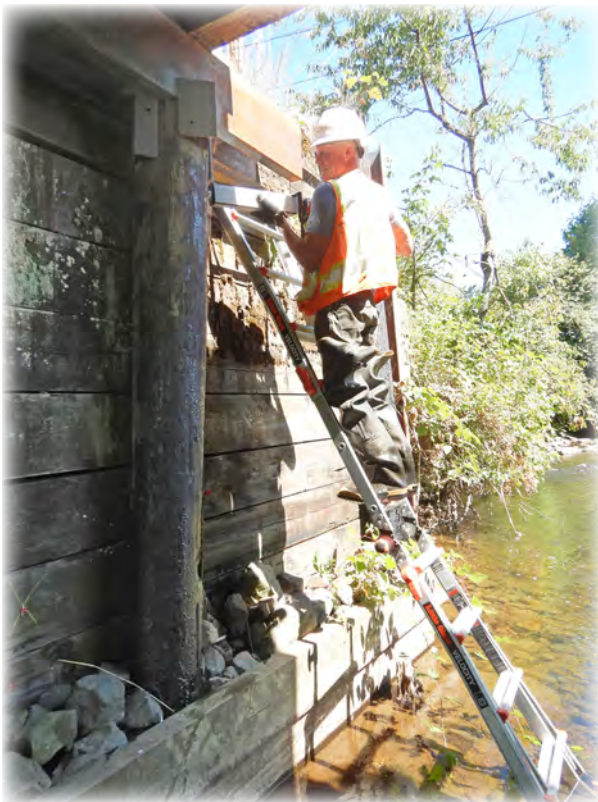
County bridge inspector drilling a timber pile at Bridge 443 to evaluate the condition and detect any decay.
