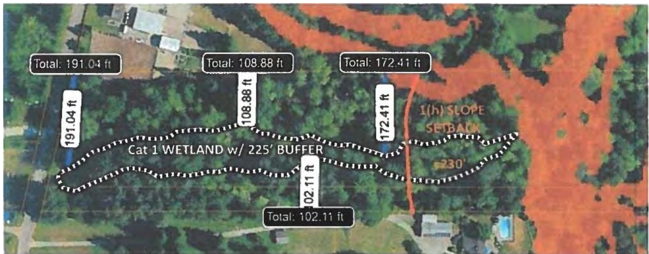
Figure 1. Mapped & observed critical areas on TPNs 280B31-01f3-001-iXI, 016-EKI: regulated steep slopes depicted in orange & approx. minimum slope setback of ≈230' depicted by orange line; wetland boundary depicted in black/white. Afl locations approximate. Image Source: Snohomish County PDS
