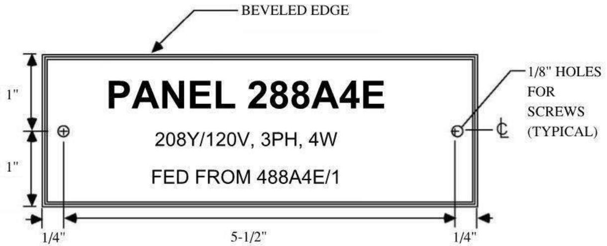
NOTE: LETTERING ON FIRST LINE IS 1/2" HIGH. ALL OTHER LINES OF LETTERING ARE 1/4" HIGH WITH 1/4" SPACING BETWEEN ALL LINES.
