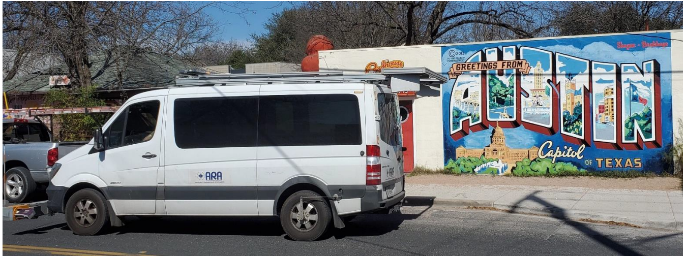
Figure 2: One of ARA’s LCMS based Pavement Evaluation Vans
